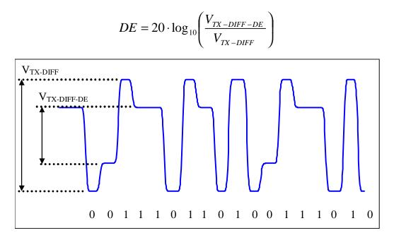
Figure 50. Differential transmitter post-cursor de-emphasized waveform
