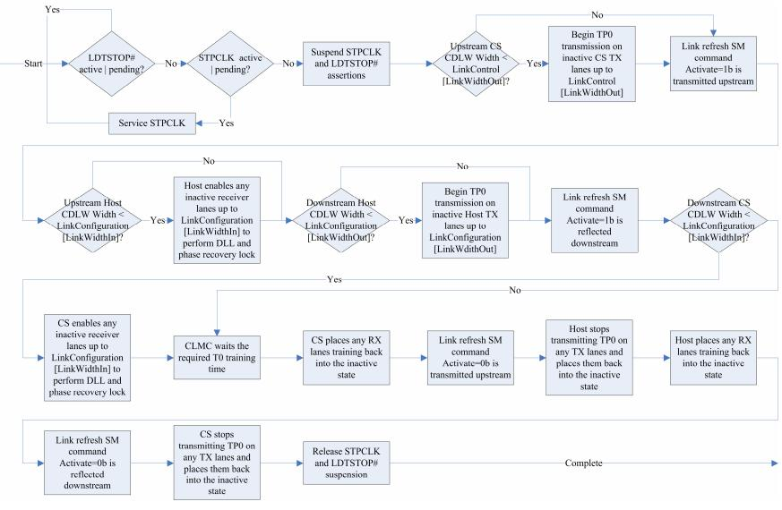
Figure 11. CLMC Sequencing Diagram for CILR
