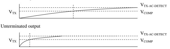
Figure 18. AC Detect Timing
