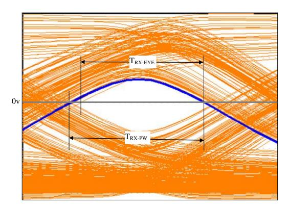
Figure 59. Receiver cumulative eye showing min-pulse width
