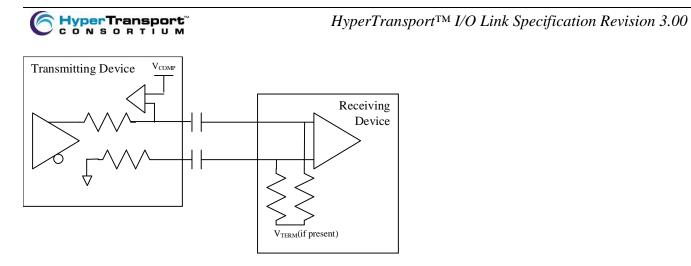
Figure 17. AC Detect Circuit
