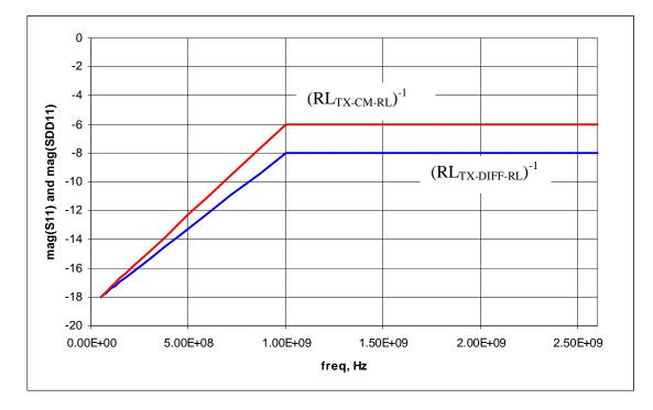
Figure 49. Transmit return loss mask
