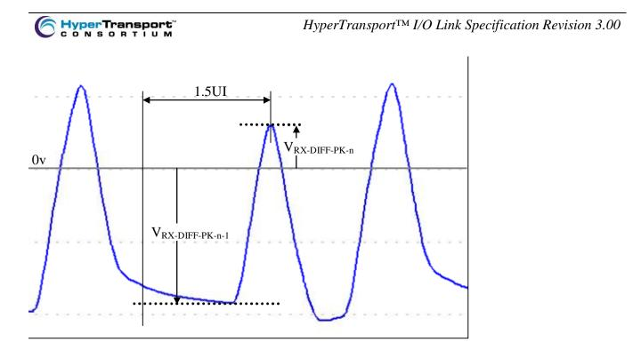
Figure 60. Receiver adjacent bit ratio
