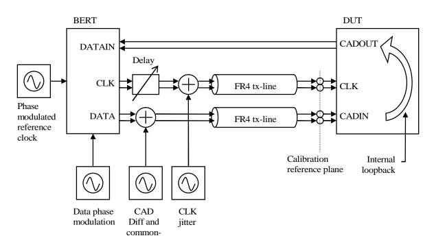
Figure 62. Receiver input compliance test setup
