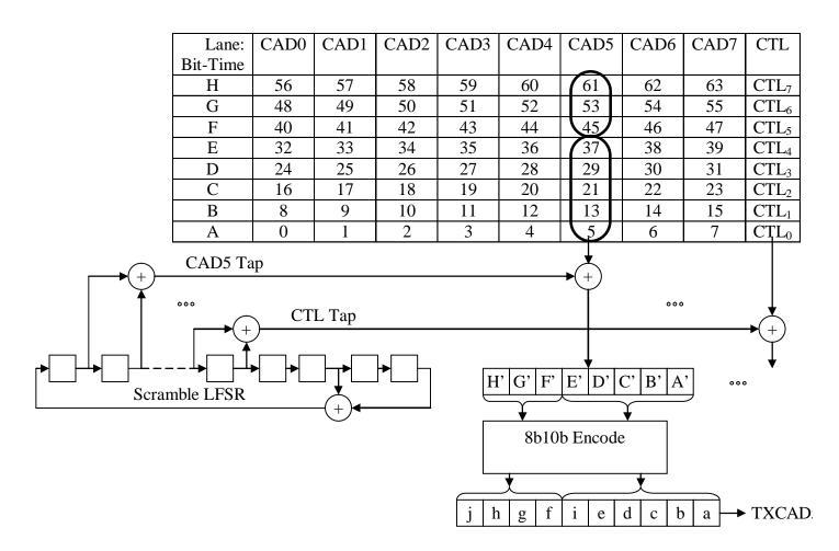
Figure 3. Gen3 Transmitter Order of Operations
