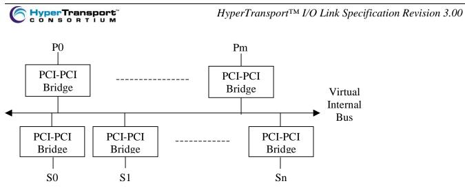
Figure 28. Logical Model of a Switch
