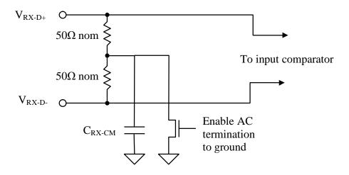
Figure 58. Receiver input termination
