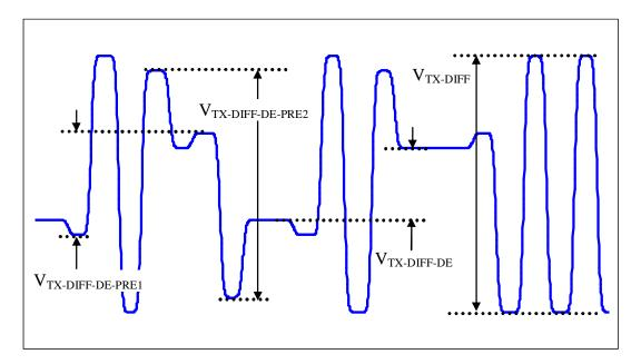
Figure 51. Transmit with pre- and post-cursor de-emphasis
