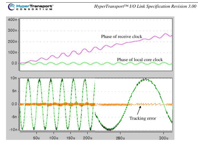
Figure 64. Phase tracking across receiver sync-fifo
